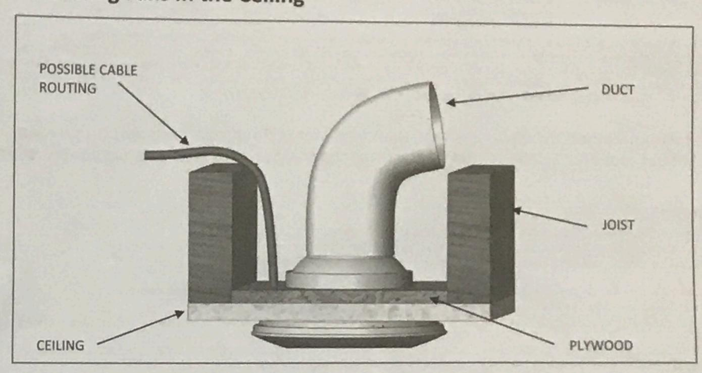
When recessing fans in the ceiling, a plywood support (min 18mm thick) should be mounted between the ceiling joists. Fans should not be fitted to unsupported plaster board.
