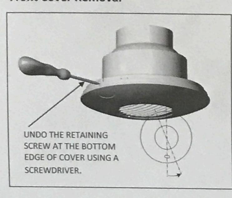
The front cover fan has a bayonet type fitting. To remove, undo the retaining screw at the bottom edge of the cover using a screwdriver, then rotate the cover a few degrees anticlockwise and remove. To refit, reverse the above procedure.
